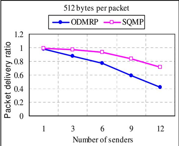
Fig.6: Effect of PDR for 512-bytes packet size
