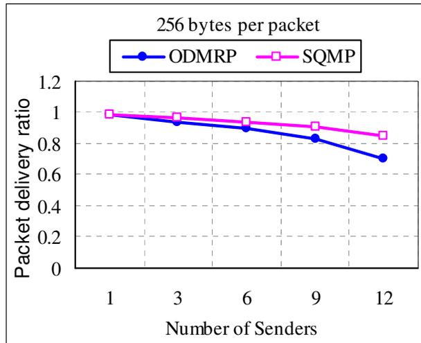
Fig.5: Effect of PDR for 256-bytes packet size
