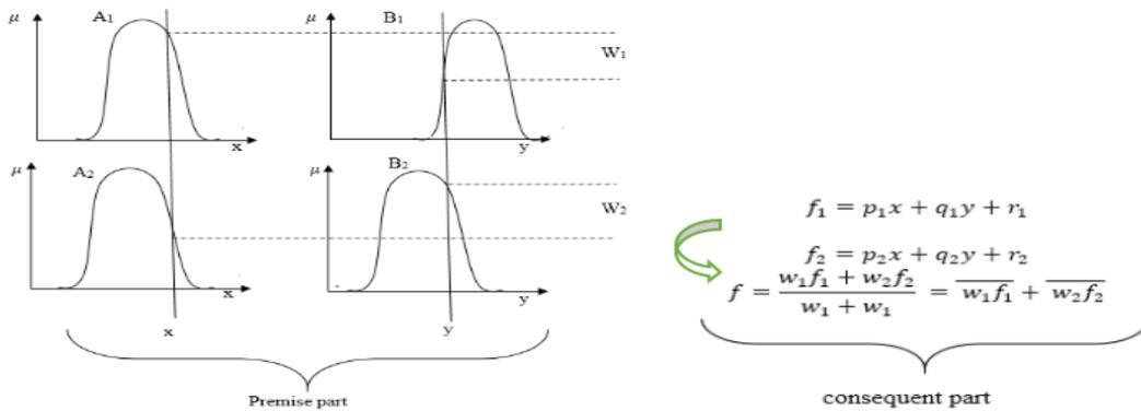
Fig. 2: Two-input first order Sugeno fuzzy model
