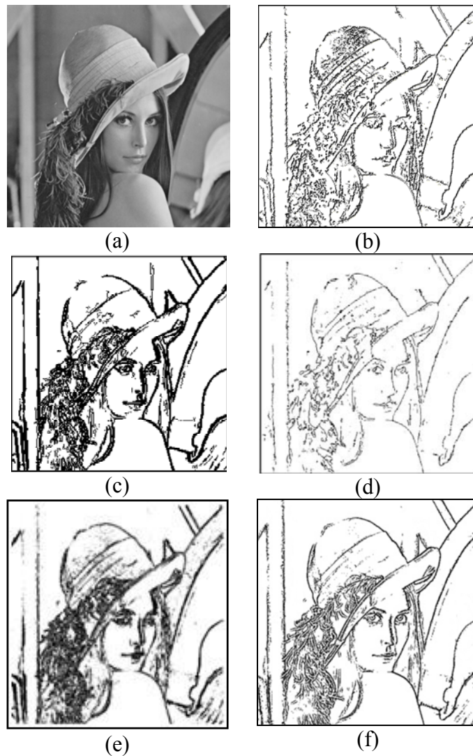
Fig. 16. The original image, (b) Fuzzy edge detector applied to the image, (c) ACO-based edge detector applied to the image (d) Neural Network edge detector applied to the image, (e) GA-based edge detector applied to the image, and (f) Universal Gravity edge detector applied to the image.
