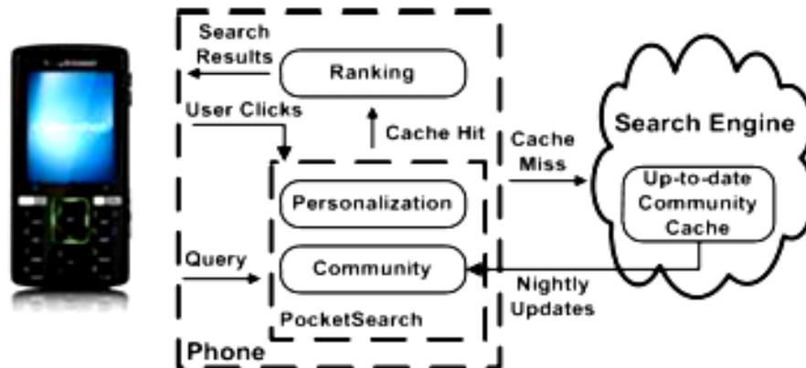
Fig. 4: Pocket Cloudlet Architecture by Koukoumidis [14]
