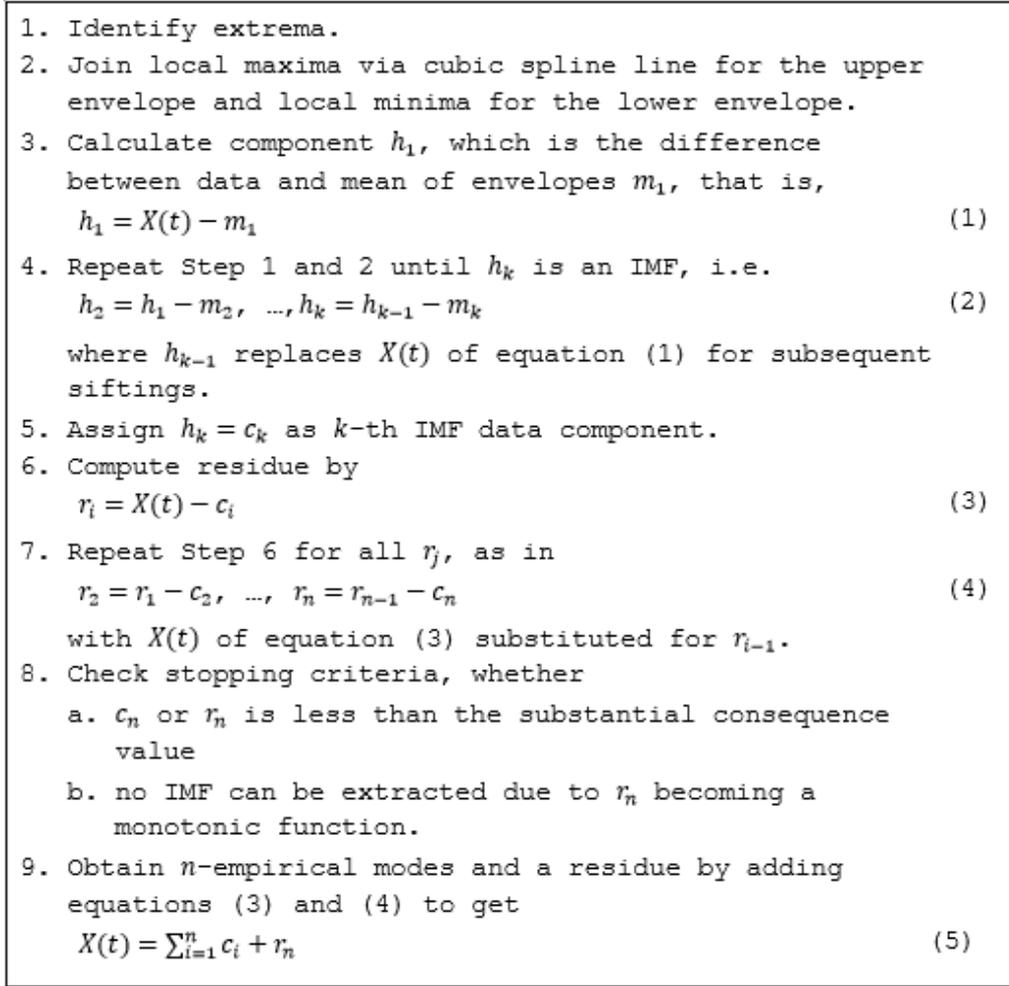
Fig. 2: Sifting process of EMD
