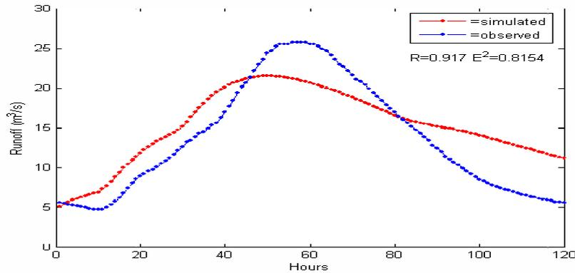
Fig. 7: Comparison between observed storm hydrograph and optimal simulated storm hydrograph using SCE
