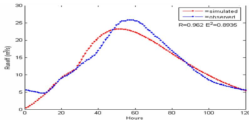
Fig. 6: Comparison between observed storm hydrograph and optimal simulated storm hydrograph using PSO
