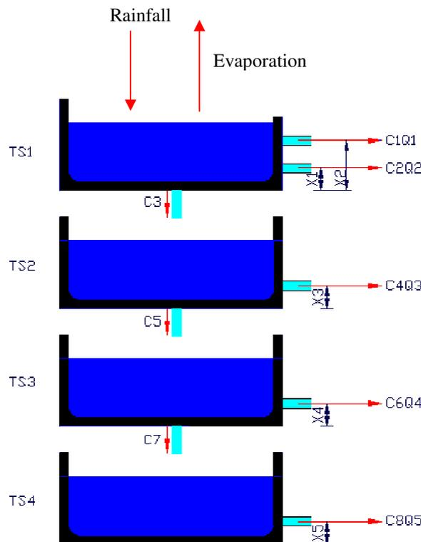
Fig. 5: Schematic of Tank Model used in this study
