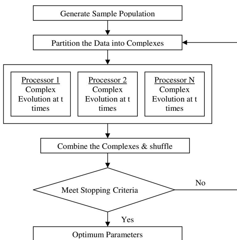
Fig. 4: SCE Calibration Process
