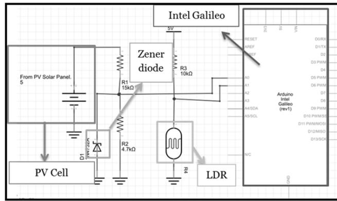
Fig. 3: Sensor Node Circuit Connection
