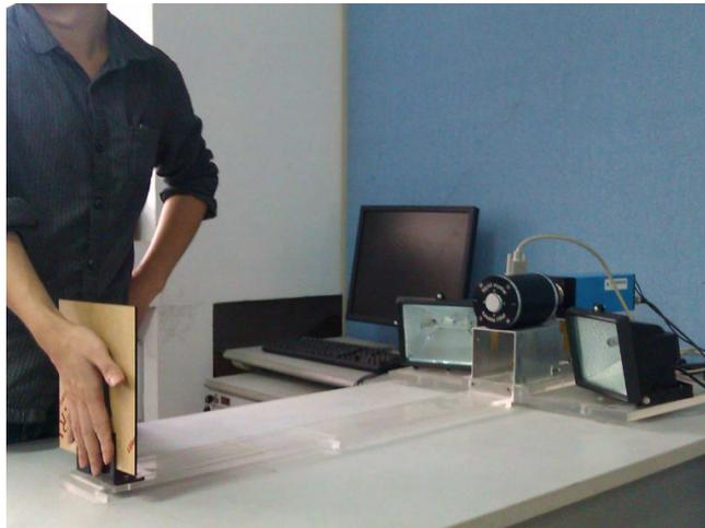
Fig 1: PUHSPD Palm Vein recognition system setup [29]
